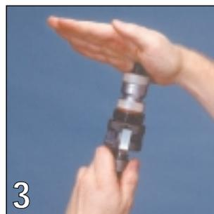
Press the cap slightly with the ball of the hand to release the pulling bolt and bring the thread shaft into the home position.
