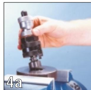
The thread of the bore hole must not be damaged. If necessary, rethread with a suitable screw tap. Grasp the *multicut*\* at the base part and the thrust piece. Screw it into the bore hole.
